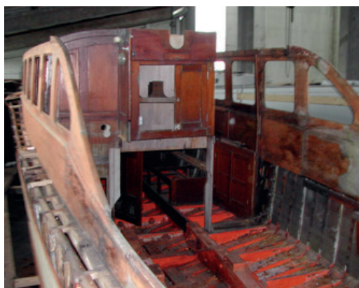
Before Stripping. Everything out. Roof, bulkheads installations damaged or rotten planks and longitudinal chines
