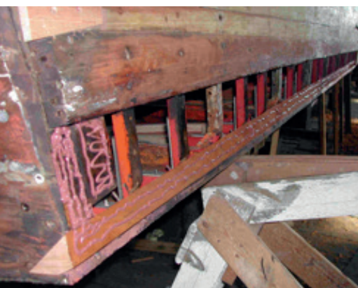
New triangular chine shifted in both sides
