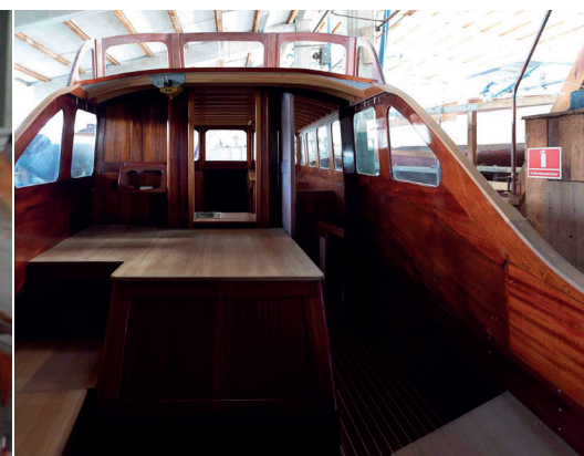
Before Stripping. Everything out. Roof, bulkheads installations damaged or rotten planks and longitudinal chines
